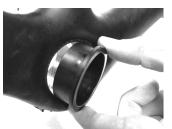
**2**. Put a tiny dab of grease on the provided Praxis Delrin PF cups. Then using your press tool, press one PF cup into each side of frame.
